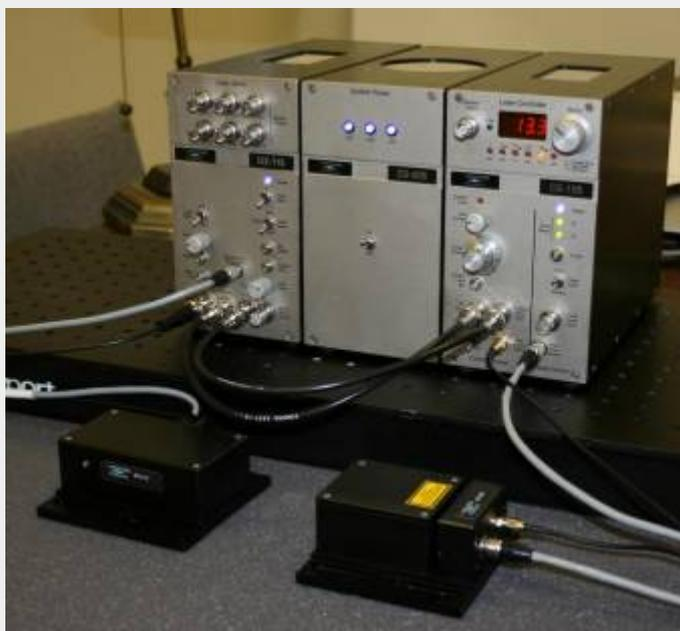
D2-110 Spectroscopy Module, connect the Hirose connector on the free end of the cable to the Temp Cntl Hirose on the D2-125-T.
