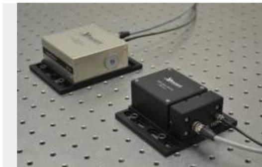
D2-100 Laser and D2-210 Spectroscopy Module on optics table
