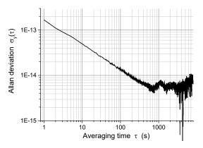
The figure shows a typical Allan Deviation (ADEV) plot for a  $Stabi\lambda aser\ 1542\epsilon$
